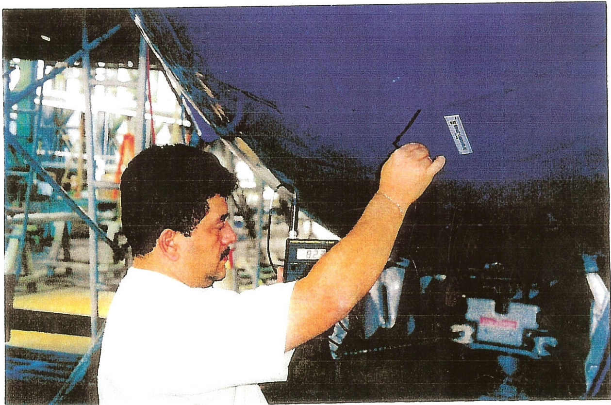
Measurement of paint thickness on Boeing 737 aircraft at repair station using digital eddy current thickness meter.
